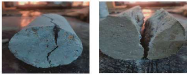
Fig. 4 Cylindrical tested specimens for split tensile strength
